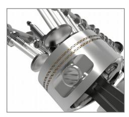
2. Oil flows through the oil ring to lubricate the piston and parts from the inside, which forms a thin film around the cylinder wall.
